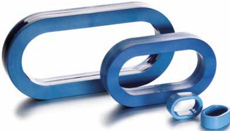
High-frequency common-mode core filters reduce electromagnetic interference and eliminate bearing damage by electrical discharge.
